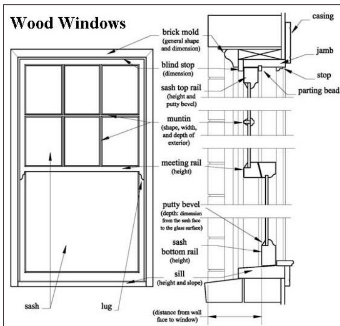
Elements of wood windows (Diagram: NPS.gov).
