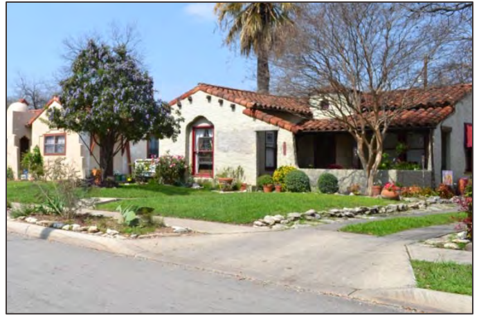
Typical front yard, Monticello Park Historic District. Note the berm in the lawn, the step in the front walkway, and the driveway with two concrete runners and a grass median.
